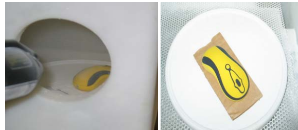
APPLY POWDER COATING TO HOT PART
