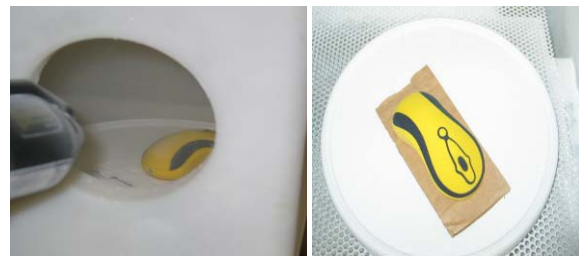
APPLY POWDER COATING TO HOT PART
