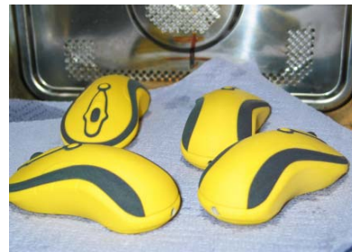
CURE PARTS IN CONVECTION OVEN
